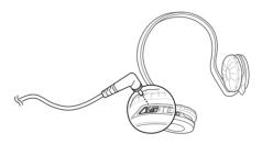
2 Plug the adapter into an electrical outlet. The red indicator light turns on. When the battery is fully charged, the indicator light changes to blue.
